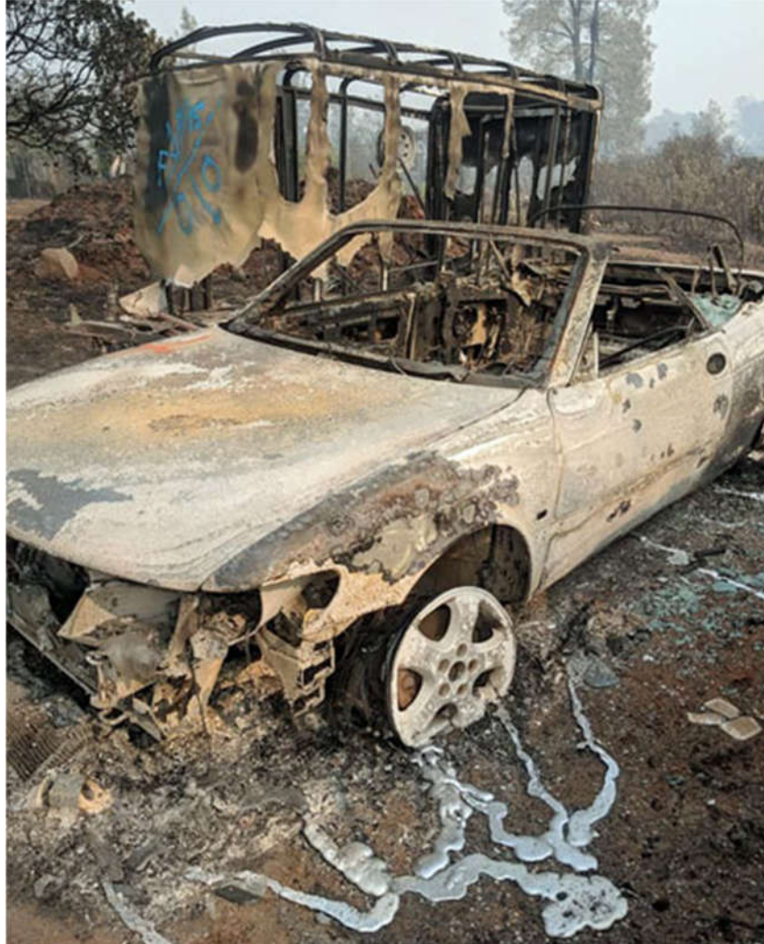
Car and Melted Aluminum Wheels Photo by RMRU Ray.
