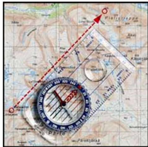
Place the compass on the map with the edge of the compass along the desired line of travel.
