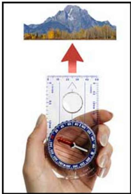
Hold the compass in your hand and turn yourself until the red end of the compass needle (North) coincides with the red arrow in the bottom of the compass housing. The front of the compass with the direction of travel arrow is now pointing towards your destination. The reverse can be done to determine the bearing based on a particular object.
